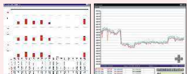
Periodic measurement of basic power quality parameters (U, I, P, Q, S, PF, etc.) with harmonics analysis performed with MI 2092 Power Harmonics Analyser .
